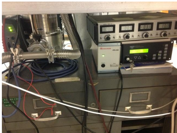
Figure 33: From left to right: Turbo pump and its respective pressure valve, Mass Flow controller sitting on top of Pressure Controller.
