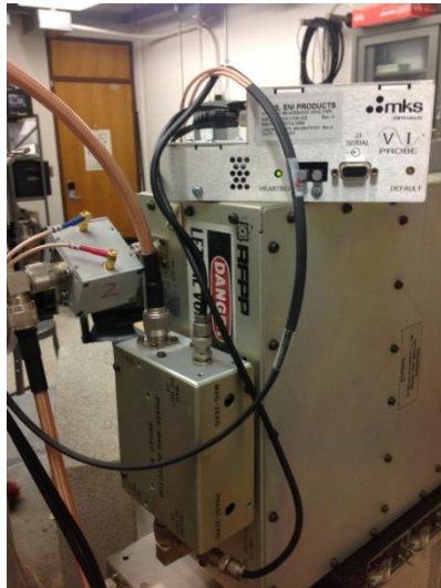
Figure 29: Alternate view of the Matching Network to show Bird Probe throughput and its connection to the analyzer.
